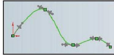
(-) Sketch5 is the sketch of a Spline. Splines are used to sketch curves that have continuously changing shape. Splines are defined by a series of points between which the SolidWorks software uses equations to interpolate the curve geometry.
